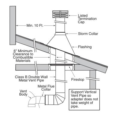
Figure 14. – Typical Metal Vent Pipe Installation - U.S. (Vertical – Negative Pressure)
