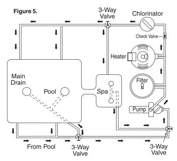
Install the chemical feeder downstream of the heater. Install
