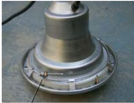
Spring clamp: Remove nut and screw
